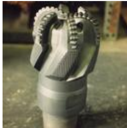
Figure 18: Shorter gauge section improves directional control, while longer improves hole concentricity.
